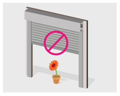
Make sure there are no obstacles in the path of the rolling shutter while the shutter is in operation.
