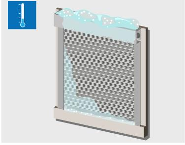
During cold weather, the curtain can freeze, either inside the housing or onto the rails. Do not use the shutter, leave in current position and avoid any forceful operation. Wait until rolling shutter is defrosted. Then it can be used again.
