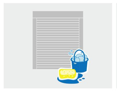
To ensure the longevity of your rolling shutter, we recommend periodic cleaning of the surface areas. Use a mild detergent and hose off (Do not pressure wash).
