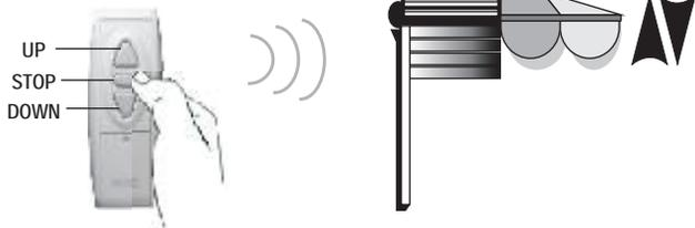
2) Check direction of operation. The DOWN button must correspond to DOWN on the motor. In the case of an awning, it will open or extend the awning. If the direction is wrong, press the STOP button on the transmitter until the motor jogs briefly UP and DOWN (approx. 5 seconds) and then release. Verify that the direction has changed and now corresponds to the transmitters UP and DOWN buttons.
