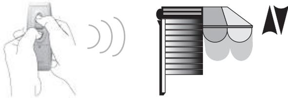
1) To assign the transmitter to communicate with the motor's receiver, push the UP and DOWN buttons on the transmitter SIMULTANEOUSLY and release the buttons after the end product jogs briefly UP and DOWN indicating the transmitter can now operate the motor for programming. The motor will now operate in a momentary fashion.
